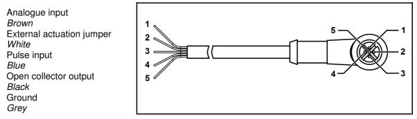
Fig. 5: RC cable pins
