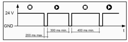
Fig. 21: Start/Stop pulse actuation
