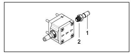
Fig. 12: Internal thread NPT 1/8"
