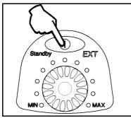
*Fig. 14: Starting / stopping the pump*
