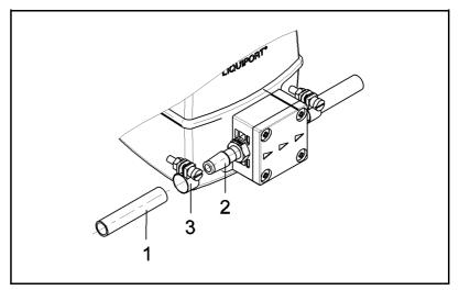
Fig. 11: Hose connector ID 8mm or ID 12mm
